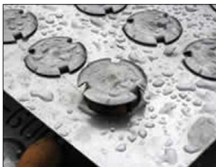
This is a typical valve tray (Fig. 3).
